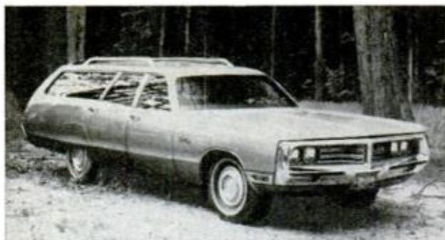
CHRYSLER TOWN AND COUNTRY wagons have new auto-lock to lock tailgate door when ignition is on
